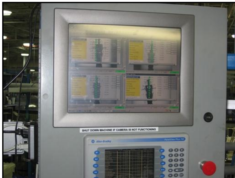
(Vision System for 100% verification check of valve core functionality)
